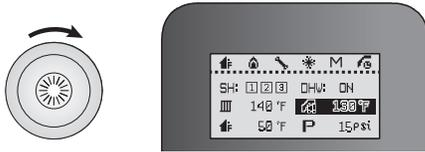
3. Press the Command dial (⊙) to select the DHW temperature (150°F). The highlighted section will flash.
